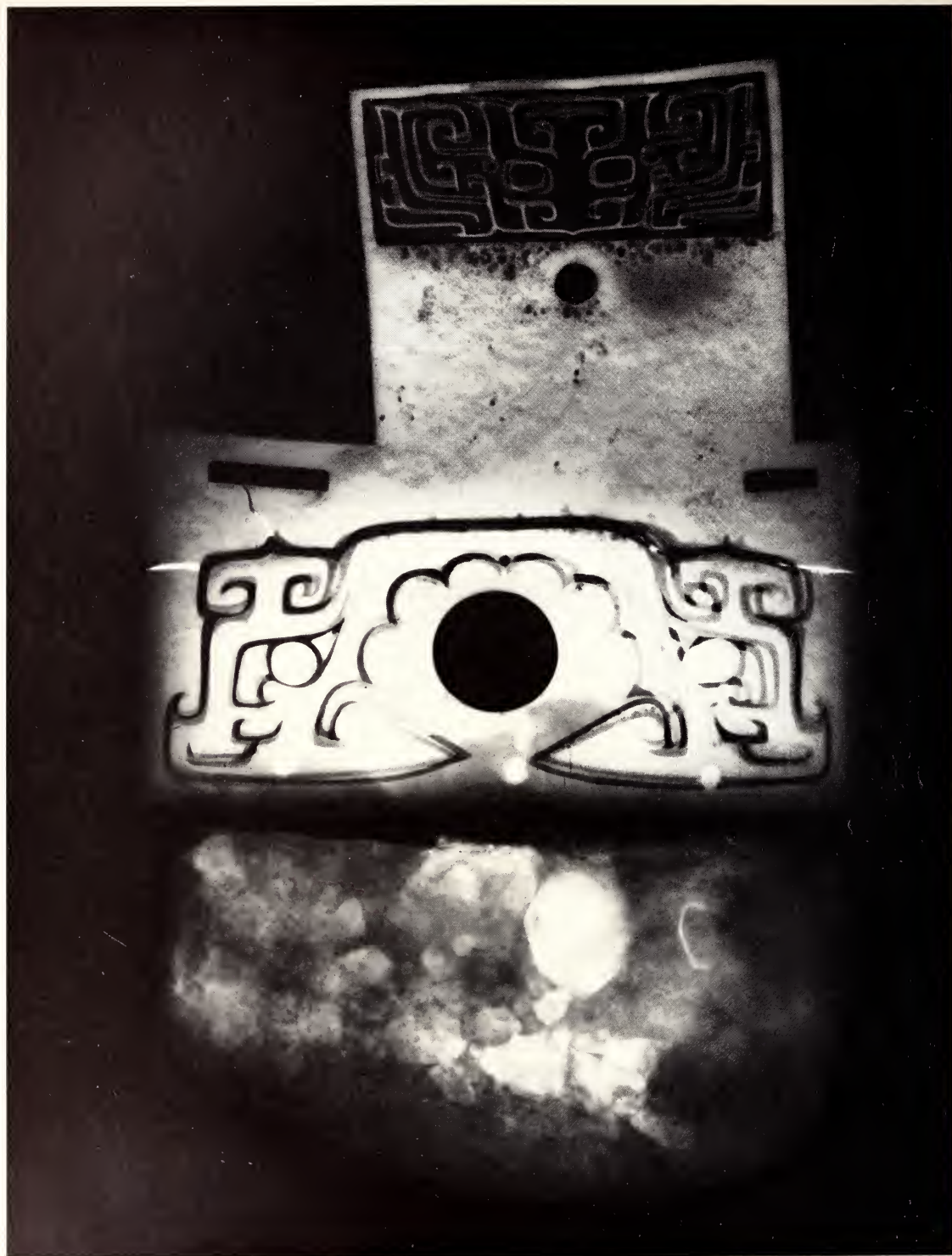
FIG. 5.—34.10. Radiograph of bronze broad axe. The view reveals that the bronze head had previously been broken into three pieces and joined with solder. It also shows three spots of high density along the ferrule edge which were later revealed to be, not rivets, but cast-in cross bars made to secure the iron blade to the bronze head. They indicate also that the bronze head was "cast-on" to the iron. Since the iron blade is almost completely converted to oxide, it hardly shows in the original radiograph, and its appearance has been enhanced photographically here. Radiograph taken at 150 Kv, 10 Ma, distance from target 76 cm.; developed in Eastman Kodak Microdol developer. Courtesy, U.S. Naval Ordnance Laboratory, White Oak, Silver Spring, Maryland.
